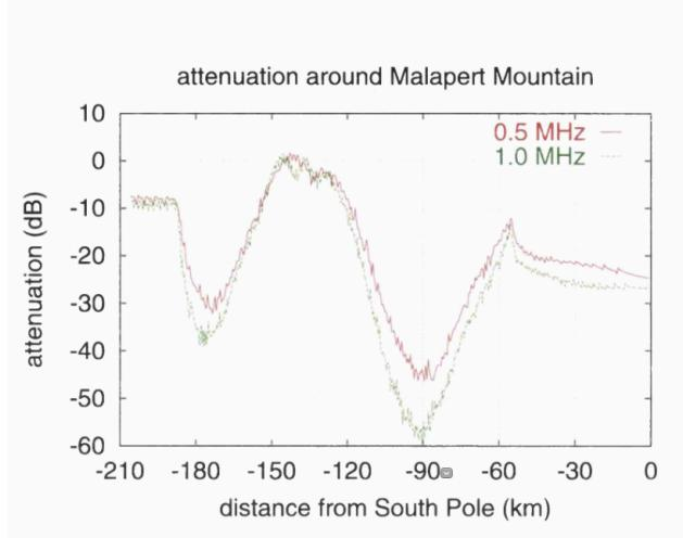
Figure 1: Simulations show that terrestrial radio waves, even at very low frequencies, would be attenuated by 5 orders of magnitude in the region directly beyond Malapert Mountain. Taken from [5].
